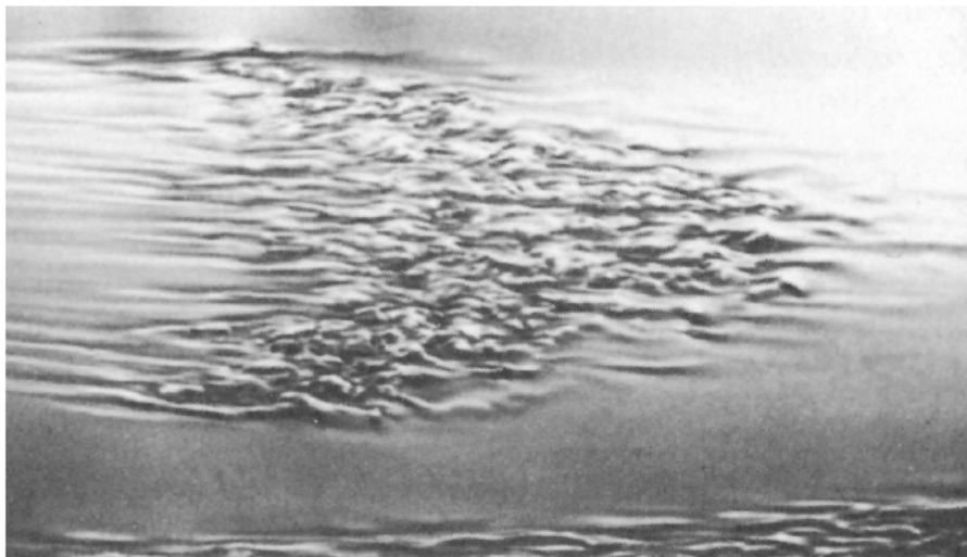
■ FIGURE 4.13 Turbulent spots and the transition from laminar to turbulent boundary layer flow on a flat plate. Flow from left to right. (Photograph courtesy of B. Cantwell, Stanford University.)
